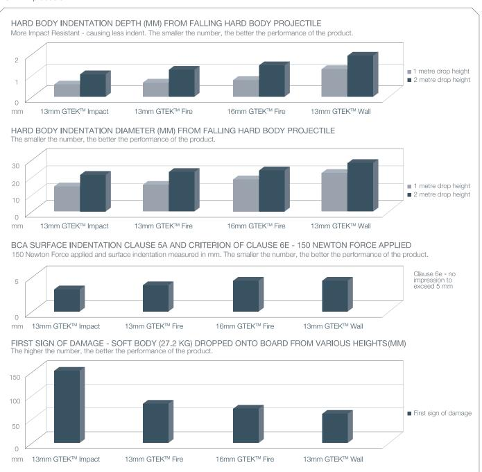
$GTEK^{TM}$  Impact is not intended to withstand deliberate damage or to be installed in areas where heavy moving machinery such as forklift trucks are used.
