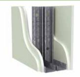
STEEL STUDS AT 600mm MAX CENTRES Side 1 1 x 13mm GTEK™ Total Plus Side 2 1 x 13mm GTEK™ Total Plus
