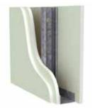
STEEL STUDS AT 600mm MAX CENTRES Side 1 1 x 13mm GTEK™ Total Plus Side 2 2 x 13mm GTEK™ Total Plus
